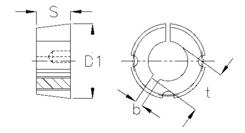
$\begin{array}{lll} b & = 1/4" \\ Bore & = 1" \\ Bush type & = 1310 \\ D1 & = 50,5 \\ S & = 25,4 \\ Screw size & = 3/8 \times 5/8" \\ t & = 1 1/8" \end{array}$
